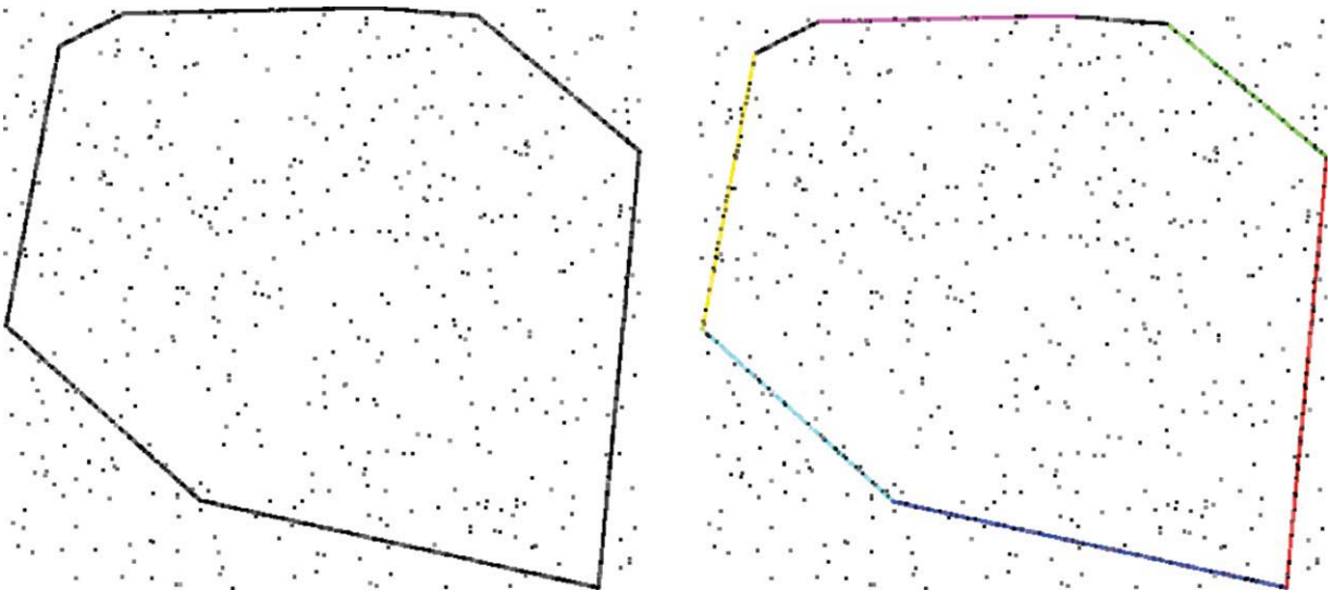
Figure 18. A polygonal contour image with noise (left), and its result after six iterations of applying our method: the optimal consensus set obtained after each iteration is in red, blue, yellow, pink, cyan, and green, respectively (right). [Color figure can be viewed in the online issue, which is available at wileyonlinelibrary.com .]
