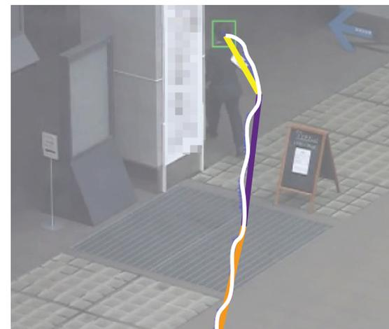
**Fig. 3** Example of polyline simplification result. Curved line shows tracking result and straight lines show simplification result.
