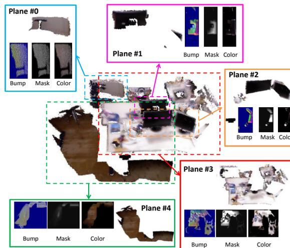
Fig.1. 3D representation for an indoor scene [11]. The target scene is segmented into multiple coplanar parts. Each segment  $S$  is modeled by the equation of the plane  $P$  that best fits the set of 3D points in  $S$ , the 2D bounding box of the projection of all 3D points in  $S$  into the plane  $P$ , and three 2D images that encode local geometry (Bump), color (Color) and confidence of measurements (Mask).
