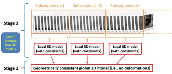
Fig.2. Overview of our two-stage strategy [12]. The first stage generates local structured 3D models with geometric constraints from short subsequences of RGB-D images. The second stage organizes all local 3D models into a single common global model in a geometrically consistent manner to minimize deformations.
