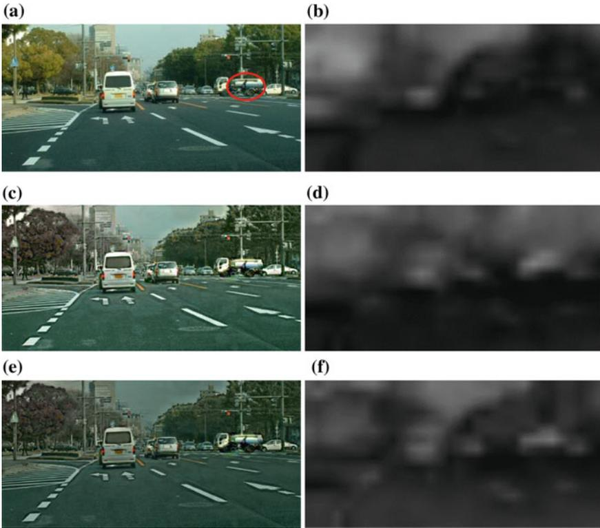
**Fig. 8.13** Examples of input image and modulated images with and without adjustment. The *red circle* in (a) is a specified region to enhance saliency. **a** Input image. **b** Saliency map of input image. **c** Modulated image with adjustment. **d** Saliency map of the modulated image with adjustment. **e** Modulated image w/o adjustment. **f** Saliency map of the modulated image w/o adjustment
