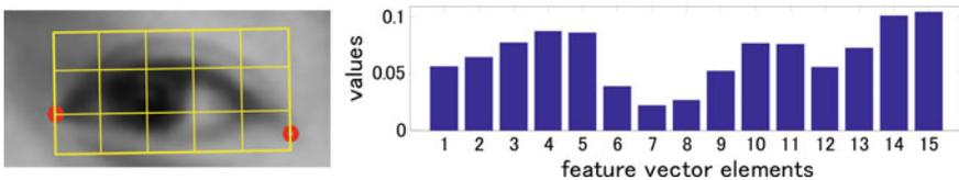
**Fig. 8.1** Eye appearance feature extraction. *Left* Illustration of eye corner detection and  $3 \times 5$  subregion division. *Right* Generated 15-D feature vector (Reproduced with permission of © 2014 IEEE [30].)
