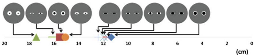
**Fig. 8.25** Errors of gaze reading for each design candidate for robot eyes. The smaller value indicate smaller error and thus a more readable gaze (Reproduced with permission of © 2013 John Benjamins Publishing Company [36].)
