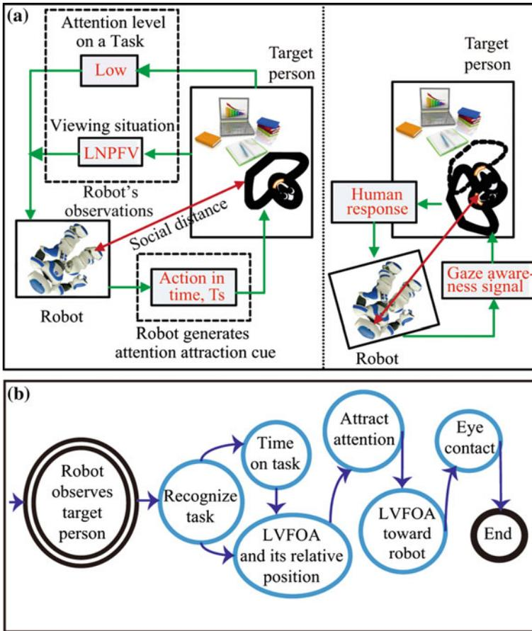
Fig. 8.19 a An abstract view of the proposed approach, and b basic steps of the proposed approach (Reproduced with permission of © 2015 IEEE [9])
