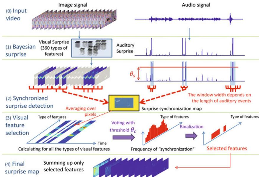
**Fig. 8.10** Framework of the proposed model (Reproduced with permission of © 2015 Springer [32].)
