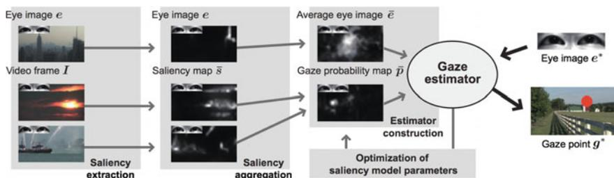
**Fig. 8.4** Illustration of the saliency-based calibration approach. The method consists of mainly four steps: saliency extraction, saliency aggregation, estimator construction and saliency model optimization (Reproduced with permission of © 2013 IEEE [44])
