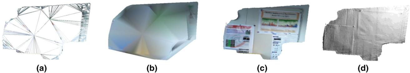
**Fig. 24** A light, yet detailed rendering of our built 3D model by taking advantage of texture mapping. **a** The geometrically simplified 3D mesh has a sparse triangulation. **b** Rendering the simplified mesh without texture mapping produces unsatisfactory results because of the loss in *color information*. **c, d** Visually detailed rendering with relighting
