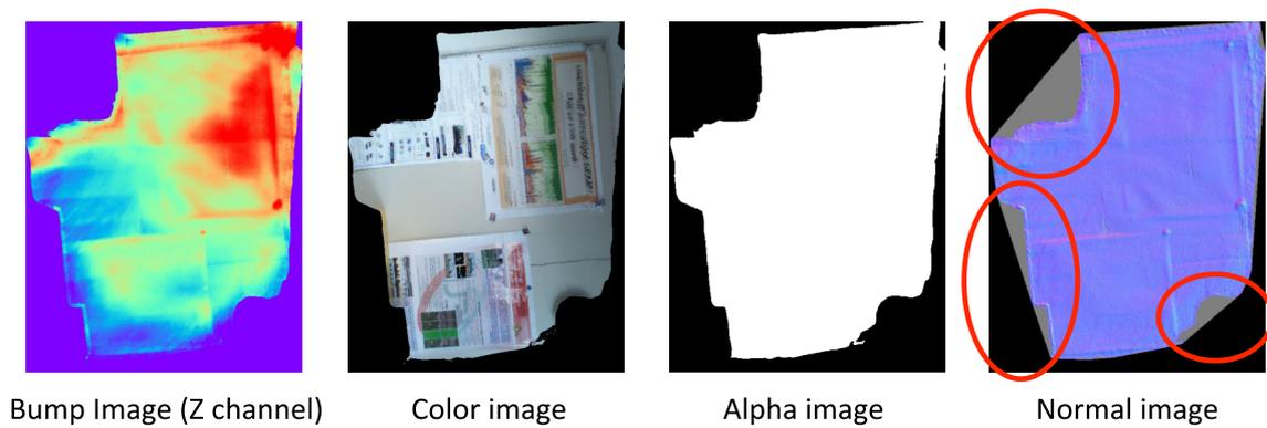
**Fig. 23** Illustration of the computed alpha and normal images for a given Color and Bump image. Empty regions in the Bump image that are covered by a *triangle* are visible in the Normal image with *grey color* (inside the *red circles*) (Color figure online)
