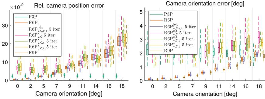
**Fig. 4.** Experiment showing the effect of the linearized camera pose which is present in all models. The further the camera orientation is from the linearization point, the worse are the results.  $R6P_{v,c,w,t}^{[v]\times}$  matches the results of R6P and so does R9P.
