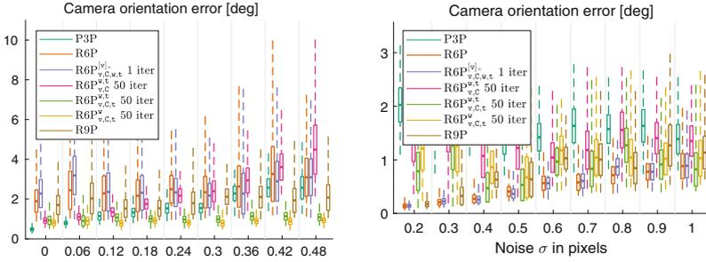
**Fig. 2.** (Left) Purely translational camera motion, increasing on the x axis. Image noise with  $\sigma$  1pix. Notice that  $R6P_{v,c,t}^w$  and  $R6P_{v,c,t}^{w,t}$  now outperform all the others. (Right) Performance on general camera motion with increasing image noise.
