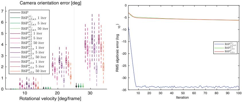
**Fig. 3.** Testing the convergence of the iterative solvers. All iterative solvers have been run with 1, 5 and 50 iterations on data with  $R = I$  and increasing RS effect (left). Convergence of the algebraic error using the three viable iterative solvers (right).
