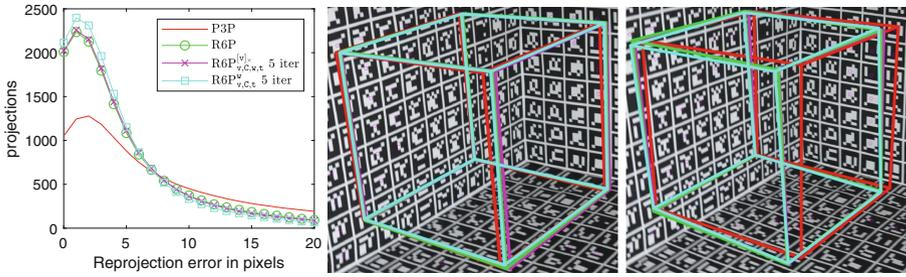
**Fig. 7.** Histogram of reprojection errors on the Aruco markers in the augmented reality experiment. The rolling shutter absolute pose solvers (R6P in magenta,  $R6P_{v,C,w,t}^{[v]x}$  in green,  $R6P_{v,C,t}^w$  in cyan) keep the cube in place during camera motion whereas P3P (red) reprojects the cube all over the place. (Color figure online)
