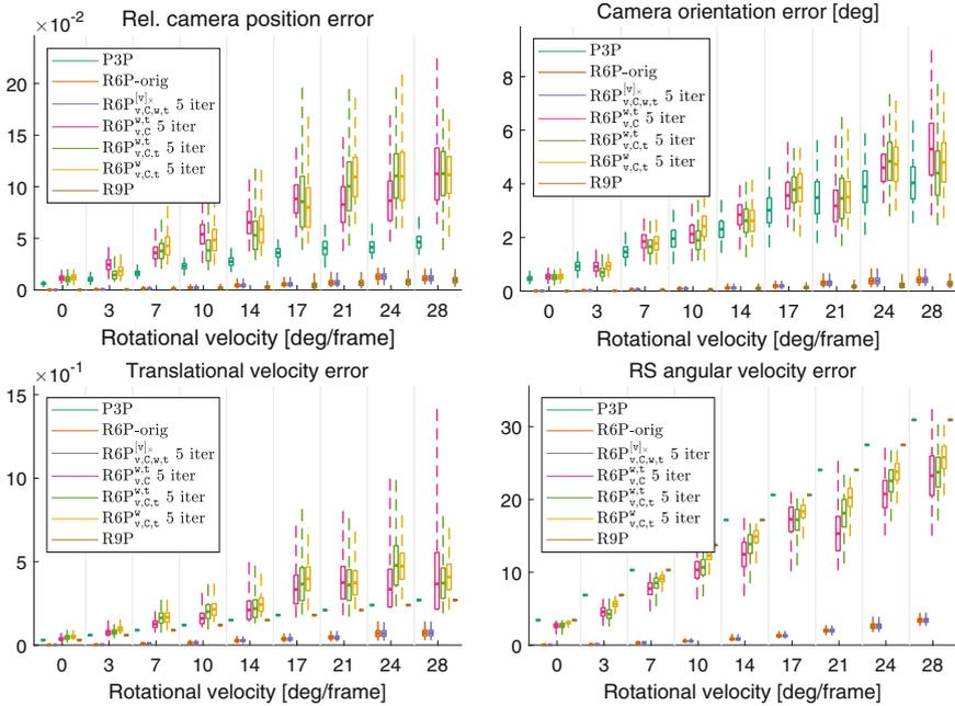
**Fig. 1.** Experiment on synthetic data focusing on the precision of estimated camera poses and velocities. Notice that the performance of  $R6P_{v,c,w,t}^{[v] \times}$  is identical to R6P. In terms of camera pose these two solvers are slightly outperformed by R9P. Other linear solvers perform very poorly in all respects.
