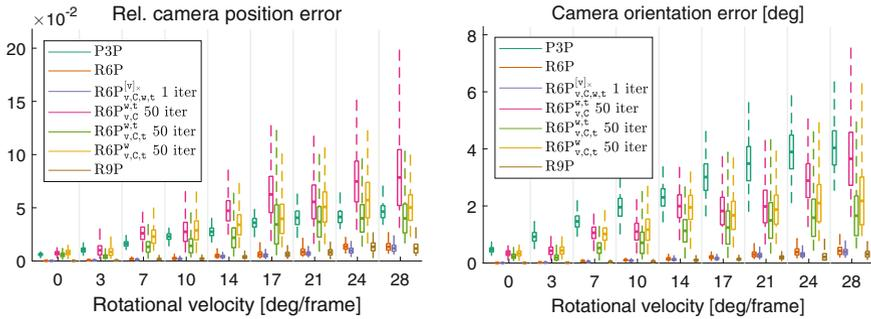
**Fig. 5.** Increasing the camera motion and estimating camera pose with all solvers being initialized with P3P.  $R6P_{v,c,w,t}^{[v]\times}$  and R9P now provide consistently excellent results, comparable or outperforming those of R6P at a fraction of the computation cost.  $R6P_{v,c}^{w,t}$ ,  $R6P_{v,c,t}^w$  and  $R6P_{v,c,t}^{w,t}$  with 50 iterations now perform better than P3P, but still not as good as the other RS solvers.
