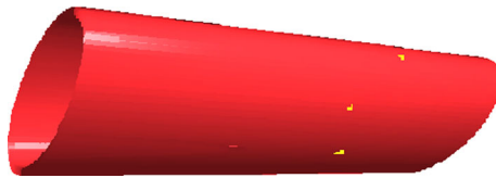
FIGURE 4. Construction of one elliptic cylinder from five points
